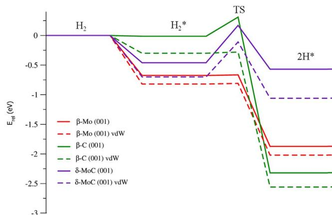
**Fig. 1.** Energy profile of  $H_2$  adsorption and dissociation including ZPE correction on  $\beta$ -Mo,  $\beta$ -C, and  $\delta$ -MoC (001) surfaces including vdW terms (dashed lines) or not (solid lines).
