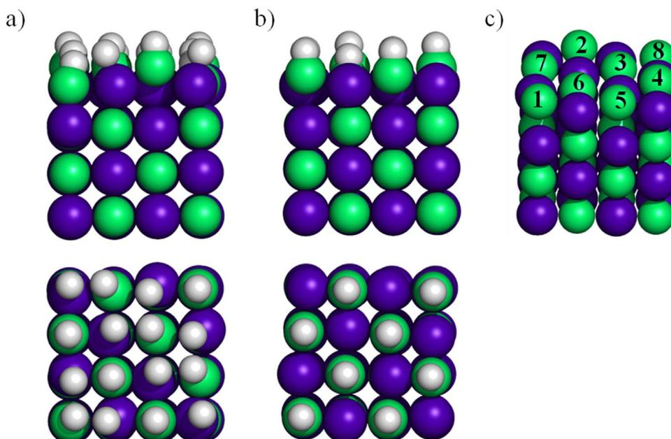
**Fig. 4.** Sketches on side view (top) and top view (bottom) of full coverage (a) and half coverage (b) hydrogenated  $\delta$ -MoC (001) surface. Picture (c) shows the C surface nomenclature of 50% hydrogenated surface used on Table 4. Sphere coloring as in Fig. 2. (For interpretation of the references to color in this figure legend, the reader is referred to the web version of this article.)
