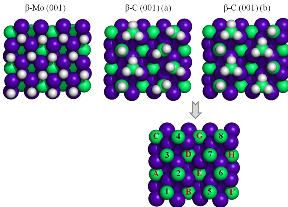
**Fig. 3.** Sketches on top view of full coverage hydrogenated  $\beta$ -Mo and  $\beta$ -C two degenerate structures. For  $\beta$ -C surface one can see the nomenclature of C atoms used on Table 3. Sphere coloring as in Fig. 2. (For interpretation of the references to color in this figure legend, the reader is referred to the web version of this article.)
