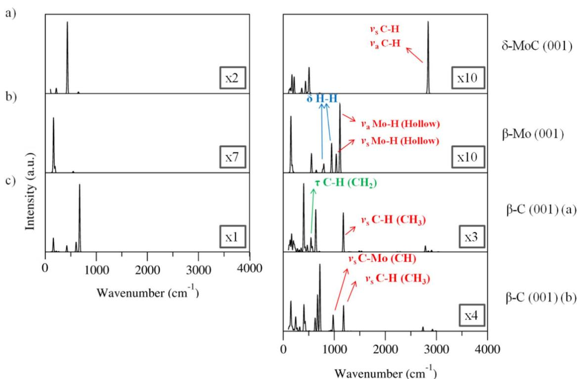
**Fig. 6.** Simulated IR spectra of bare (left) and fully hydrogenated, full coverage, (right) of  $\delta$ -MoC (a),  $\beta$ -Mo (b), and  $\beta$ -C (c) (001) surfaces. The intensities have been enlarged by factor shown on the respective panels in order to improve the visualization.
