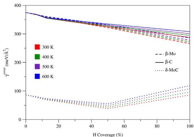
Fig. 5. Plots of surface free energy at H coverage ( $\gamma^{\text{cover}}$ ) depending of the temperature at different H coverage at 5 atm of pressure.
