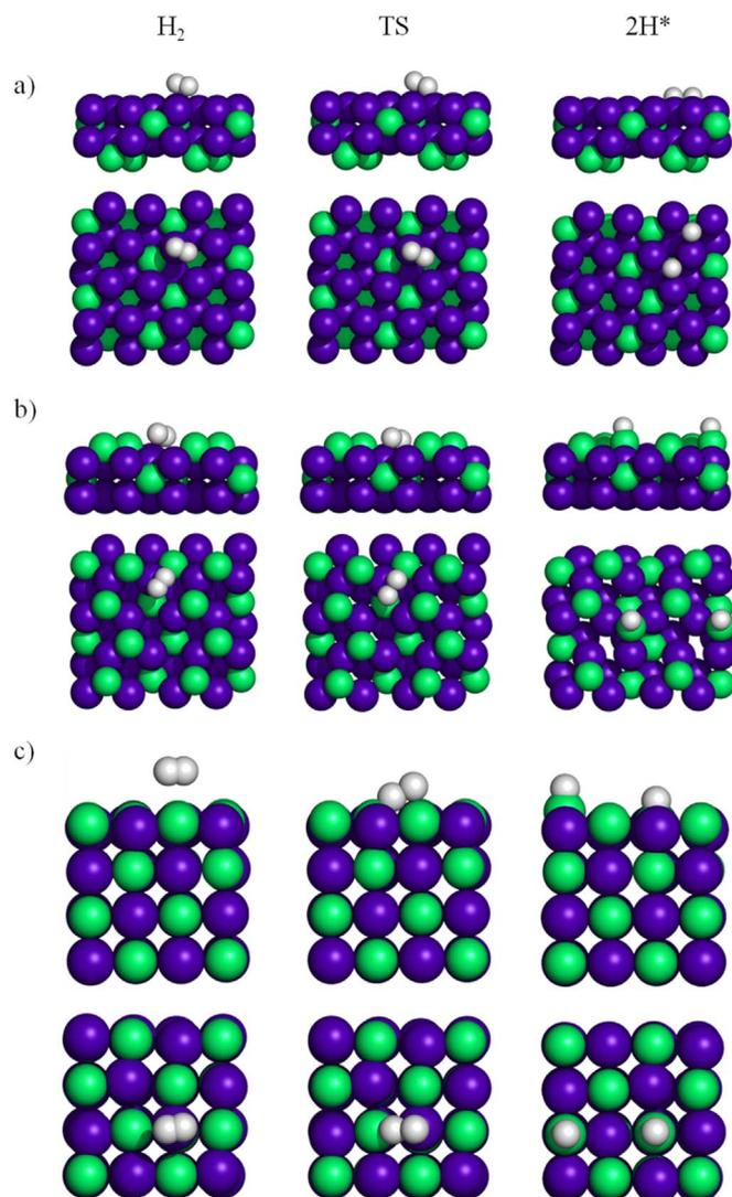
**Fig. 2.** Sketches on side view (top) and top view (bottom) of  $H_2$  adsorption (left), TS (middle), and  $2H^*$  adsorption (right) on  $\beta$ -Mo (a),  $\beta$ -C (b), and  $\delta$ -MoC (c) (001) surfaces. Pictures correspond to calculations including vdW dispersion. Violet, green, and white balls represents Mo, C, and H atoms, respectively. (For interpretation of the references to color in this figure legend, the reader is referred to the web version of this article.)
