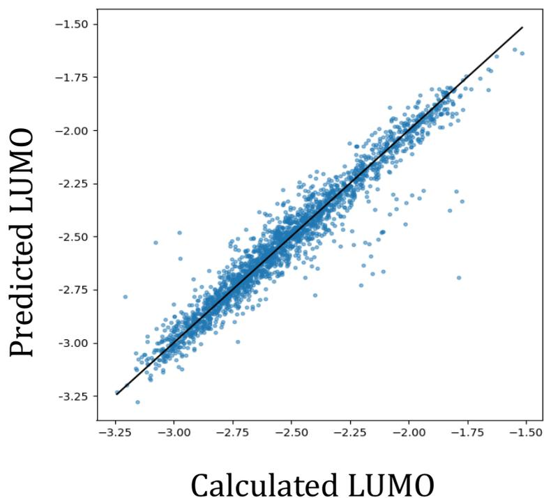
Figure 2: Predicted vs. Calculated (DFT) LUMO levels for the molecule in Fig 1. Training machine learning algorithms on this dataset will enable discovery of new polymers with optimally aligned energy levels for organic solar cells.
