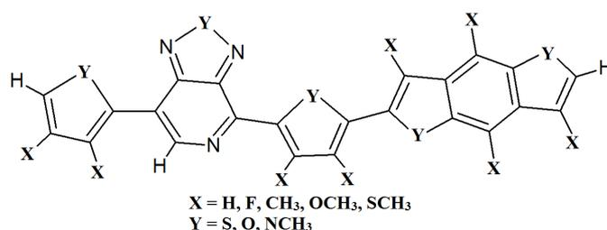
Figure 1: Example of a donor-acceptor monomer from the INKA project. Apart from varying the donor-acceptor backbone, the molecule can be functionalized by different side groups marked by X and Y. Using computational screening the structure and energy levels of a large number (>10.000) of monomers are investigated.
